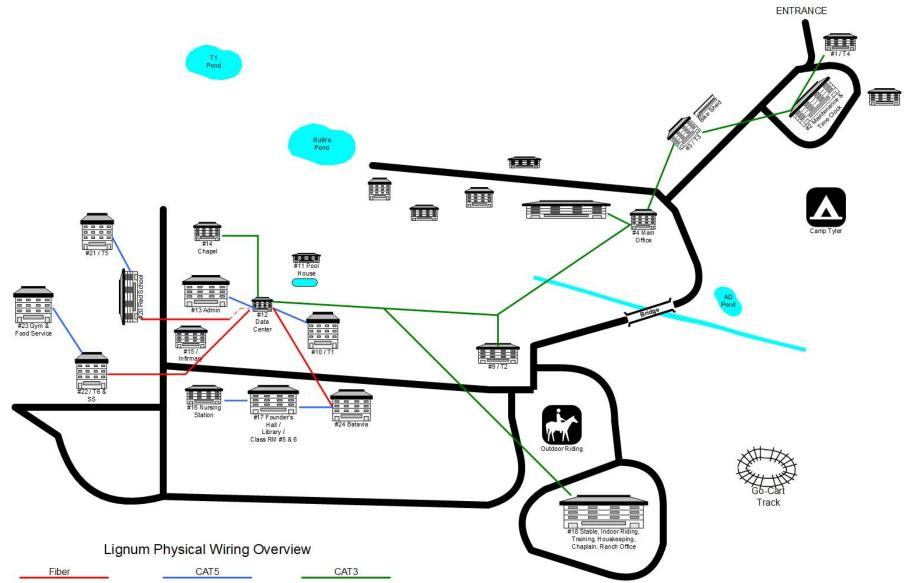
The site currently has a 4.5mbs Internet link that is shared with everyone at the location. This is being upgraded to 20mbs by April 2016. This connection comes into the admin building via bonded T1 lines. Each location that is connected via fiber has a 1gbit connection to the admin building that is shared by
